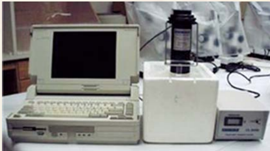
Figure 2 - Programmable Freezing Equipment
